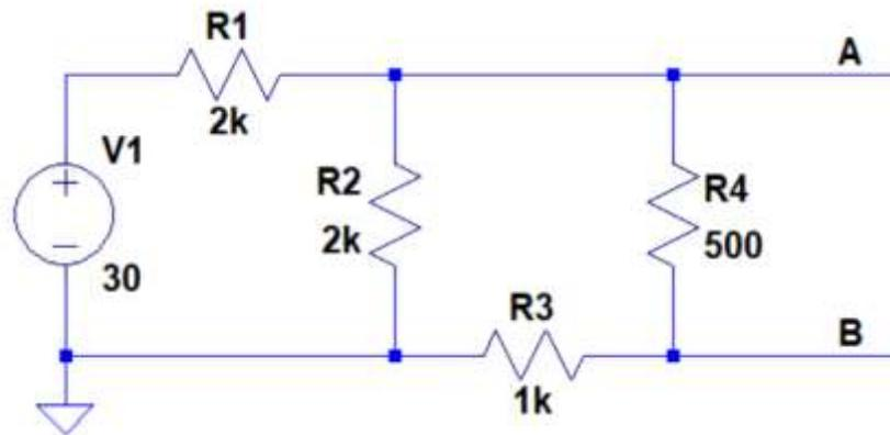
Step 1: Solve the above "Original Circuit" with a Load Resistor ( $R_L$ ) of 100ohms connected between terminals A and B. Include this hand calculated solution with the lab write-up and fill in the table at the end of the lab hand-out with  $V_{RL}$  and  $I_{RL}$ . Label this solution as Step 1.
